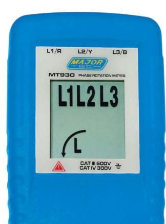
The MT930 is a compact handheld Phase Rotation indicator that has a large LCD to indicate the phase presence and rotation. Once connected to a 3 Phase power system, the meter indicates the phase sequence by displaying its corresponding phase symbol on the LCD, as well as the rotation by arrows indicating a clockwise or anti-clockwise direction. The MT930 operates from 40VAC to 690VAC.
