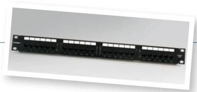
The 1100GS5 panel features a new termination manager and redesigned rear housing. The termination manager and new rear housing provide for easier, faster, more reliable terminations, and reduced variability in the placement and termination of cables to the panel.
