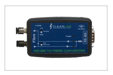
The RS485 Fibre Converter provides surge protection for any RS485 bus carrying data signals from a host computer to peripheral devices. Applications include access control and monitoring systems. No setup for baud rate is required as the device is transparent to dataflow. The unit is powered from a mains adaptor and draws 50mA at 12VDC. Indicators have been provided for power, RX and TX data.
