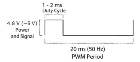
From the picture we can understand that the PWM signal produced should have a frequency of 50Hz that is the PWM period should be 20ms. Out of which the On-Time can vary from 1ms to 2ms. So when the on-time is 1ms the motor will be in 0° and when 1.5ms the motor will be 90°, similarly when it is 2ms it will be 180°. So, by varying the on-time from 1ms to 2ms the motor can be controlled from 0° to 180°
