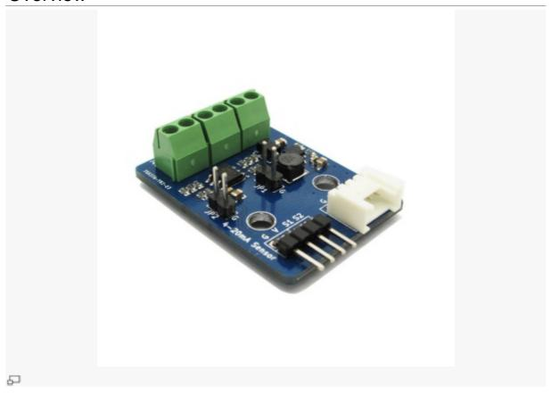
4~20mA Sensor Brick is an electronic brick module that can be used to test electronic current loop from 4mA to 20mA and support type2,3,4 current output. With a 5V to 24V DC-DC power boost convertor, its max current output can be 150mA, which can be for equipment use.
