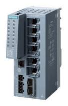
SCALANCE XC206-2SFP G (E/IP) manageable Layer 2 IE switch; IEC 62443-4-2 certified; 6x 10/100/1000 Mbps RJ45 ports; 2x 1000 Mbps SFP; 1x console port; diagnostics LED; redundant power supply; temperature range -40 °C to +70 °C; assembly: DIN rail/S7 mounting rail/wall; redundancy functions; office features (RSTP, VLAN,...); PROFINET IO device; Ethernet/IP-compliant; C-PLUG slot; default EtherNet/IP. IEEE 1588v2 PTP
