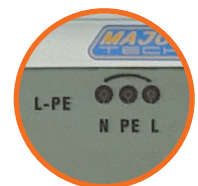
Visual indication of reversed phase and neutral wiring of socket
