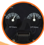
Rotary Switches for Proximity Pilot and Control Pilot States
