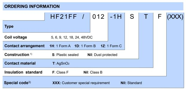
Notes: 1) Under the ambience with dangerous gas like H<sub>2</sub>S, SO<sub>2</sub> or NO<sub>2</sub>, plastic sealed type is recommended; Please test the relay in real applications.
