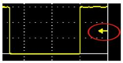
The arrow circled above is the trigger level position, and when the edge of the square wave in the above figure passes upwards through the position of this arrow, a trigger is formed (the waveform only forms a trigger when it crosses the trigger level up or down).
