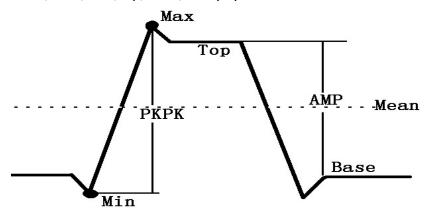
The difference between peak-to-peak and amplitude(AMP) is shown in the figure above.
