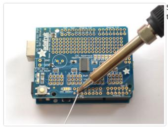
Solder each of the pins to secure the shield to the headers
