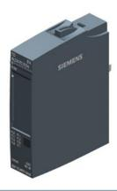
SIMATIC ET 200SP, Digital output module, DQ 8x 24V DC/0,5A Basic, Source output (PNP,P-switching) Packing unit: 1 piece, fits to BU-type A0, Colour Code CC02, substitute value output, module diagnostics for: supply voltage
