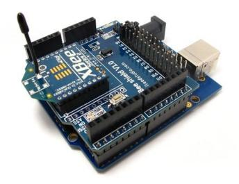
XBee Shield V1.1 is an enhanced serial port XBee module breakout board, it's compatible with Arduino and IFLAT-32, it can directly plug in with Arduino/IFLAT-32 board, and use any pin of the basic board to connect with the XBee module serial port.
