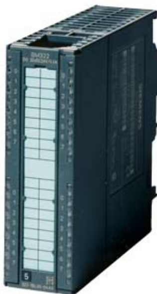
SIMATIC S7-300, DIGITAL OUTPUT SM 322, OPTICALLY ISOLATED 16 DO, 120/230V AC, 1 A, 1 X 20 PIN
