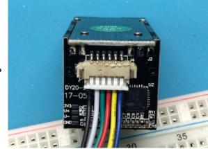
If your sensor has different wires, The first wire from the left should be the black wire ground, then the two data pins, RX is the white wire, TX is the green wire then the red power wire. You'll have to cut, strip and solder thicker gauge wires to the current wires.
