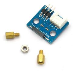
3. Sensor is located on the edge of PCB to facilitate detection.
