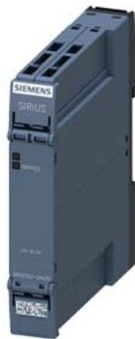
thermistor motor protection relay compact evaluation unit, 17.5 mm enclosure, spring-loaded terminal, 1 change-over contact,  $U_s = 24$  V AC/DC, Auto RESET, suitable for bimetallic temperature switches, supply=output voltage, 1 LED (tripped)
