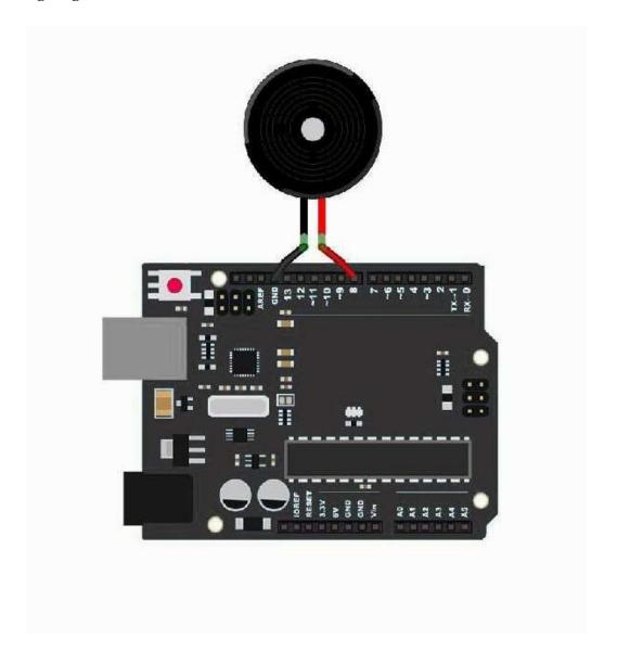
Wiring the buzzer connected to the UNO R3 board, the red (positive) to the pin8, black wire (negative) to the GND.
