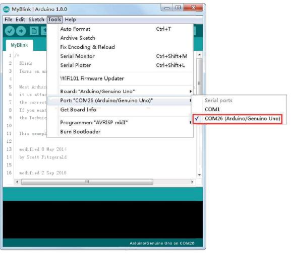
Note: The Board Type and Serial Port here are not necessarily the same as shown in picture. If you are using 2560, then you will have to choose Mega 2560 as the Board Type, other choices can be made in the same manner. And the Serial Port displayed for everyone is different, despite COM 26 chosen here, it could be COM3 or COM4 on your computer. A right COM port is supposed to be COMX (arduino XXX), which is by the certification criteria.
