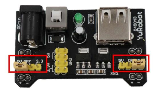
The left and right voltage output can be configured independently. To select the output voltage, move jumper to the corresponding pins. Note: power indicator LED and the breadboard power rails will not power on if both jumpers are in the "OFF" position.
