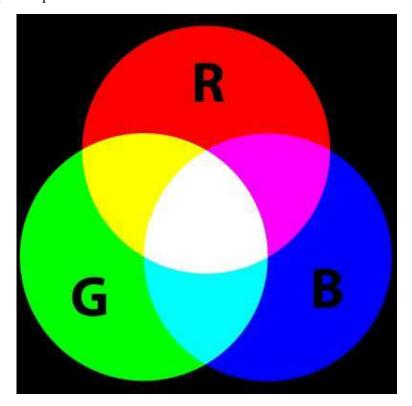
If we set the brightness of all three LEDs to be the same, then the overall color of the light will be white. If we turn off the blue LED, so that just the red and green LEDs are the same brightness, then the light will appear yellow.
