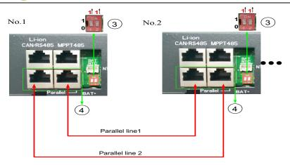
■ If there are more than two inverters parallel in your system, only two of longest distance of need to be dialed toward "on "position: 1111, and others keep off: 0101
