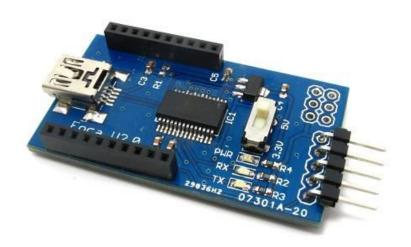
Foca V2.0 is a USB to serial UART board with XBee interface socket. It's the essential tools for establishing communication between PC and mostly MCU or use XBee. Especially, it's the optimum tool for the board which basic Arduino but without USB interface, like Sniffer Nano, Colorduino and etc.
