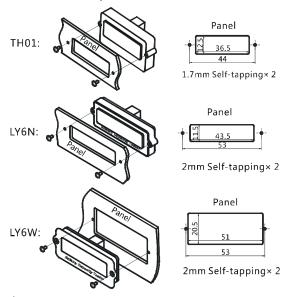
★ LY6W: First, open one rectangular orifice and two screw holes on the panel of the equipment. Then install the tester from the front of the panel, and put the shell of tester into the rectangular orifice. Finally, fix the tester with tapping screws from the front of the panel. As shown above:
