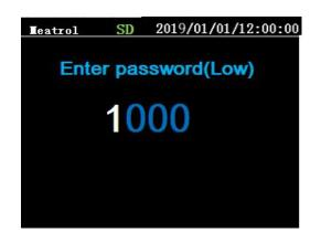
Press **Enter** ,change to next line. Press **Up/Down**,modify value on current line. Long press **Up/Down**,change display number position.
