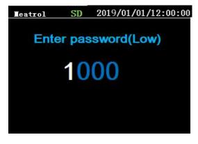
Enter "**Set**" on Menu interface. Enter Password(Low) :1000 (default) Press Up/Down to change number. Long press "Up/Down" to change display number position.
