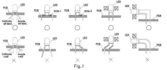
" $\bigcirc$  " Correct mounting method "imes" Incorrect mounting method
