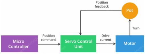
RC servo motor works on the same principal. It contains a small DC motor connected to the output shaft through the gears.
