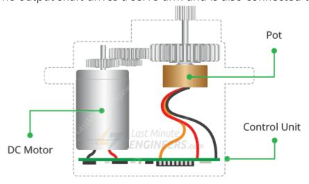
The potentiometer provides position feedback to the servo control unit where the current position of the motor is compared to the target position.
