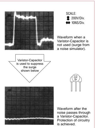
The Varistor-Capacitor is capable of removing even 1200V surges and will withstand 2000V impulses.
