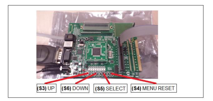
As the UP/DOWN buttons are pressed, the Explorer 16 LCD screen will refresh and change the position of the selection cursor (">") in a list of available sensor types. The output to the serial monitor will also change to indicate the current sensor type which can be selected by pressing the (S5) SELECT button. Once the user selects a sensor from the menu, the sensor data output will be displayed and updated on both the LCD and serial monitor.
