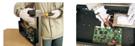
1. Install fixed screw for HDD 2. HDD data line and power line connection
