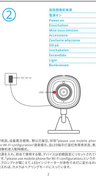
After powering on, the device is reset by default during the first use. The camera entered the pairing mode successfully when you hear the voice prompt: "please use mobile phone for Wi-Fi configuration" and see the LED indicator turns to solid red.
