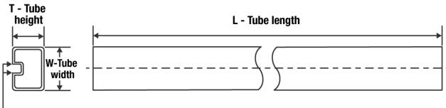
B - Alignment groove width
