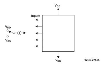
Measure inputs sequentially to both V<sub>DD</sub> and V<sub>SS</sub>. Connect all unused inputs to either V<sub>DD</sub> or V<sub>SS</sub>. Measure control inputs only.
