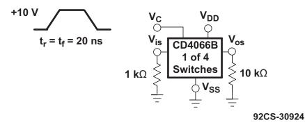
All unused terminals are connected to V<sub>SS</sub>.
