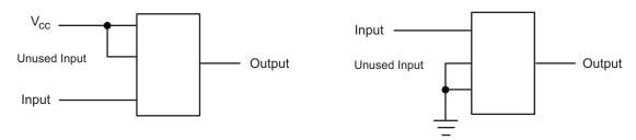
Figure 20. Diagram for Unused Inputs
