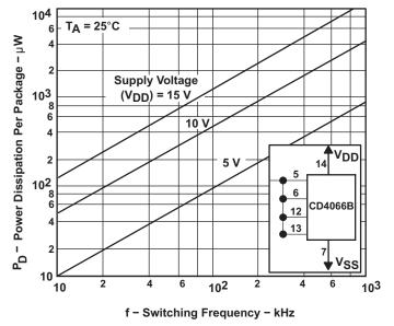
Figure 19. Power Dissipation vs. Switching Frequency
