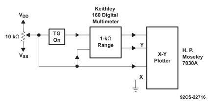
Figure 8. Channel On-State Resistance Measurement Circuit
