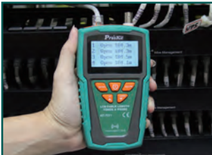
Locate break point and length measurement
