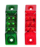
This strobe light is a visual indicator (flashes) of an alarm that has been triggered. The strobe light carries on flashing after the alarm as an event memory indicator.
