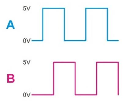
If you only wish to monitor the speed of rotation then you can use either output and simply measure the frequency. The reason for having two outputs is that you can also determine the direction of shaft rotation by looking at the pattern of binary numbers generated by the two outputs.
