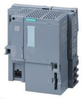
SIMATIC DP, CPU 1512SP-1 PN for ET 200SP, central processing unit with work memory 400 KB for program and 2 MB for data, 1st interface: PROFINET IRT with 3-port switch, 25 ns bit performance, SIMATIC Memory Card required, BusAdapter required for port 1 and 2
