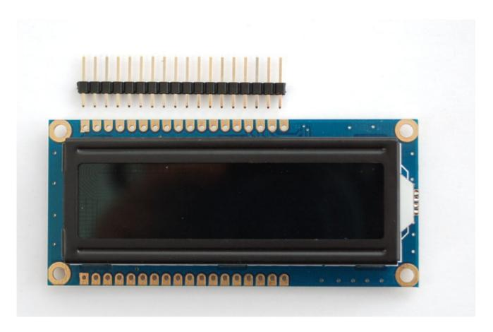
Place the header with the long side down into a breadboard. then place the LCD on top. If you're using an LCD with two rows available, make sure you're using the row that matches the image below.
