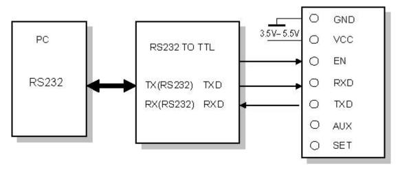
Figure 3 the connection of setting parameters
