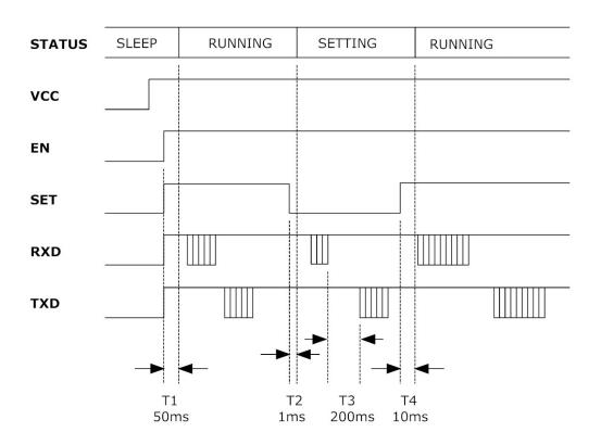
Figure 4 the figure of Setting Parameters Online
