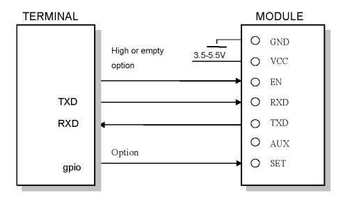
Figure 5:The Connection between Module and Terminal
