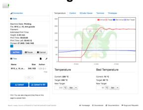
If you own a 3D printer then a Raspberry Pi is a great way to put it on your network so you don't need a **dedicated** computer. OctoPrint will connect to most 3D printers and control them over the network. The software will allow a user to upload files for printing or prepare and modify them from any computer. Prints can be started and monitored with a camera so you don't need to stay with the printer.
