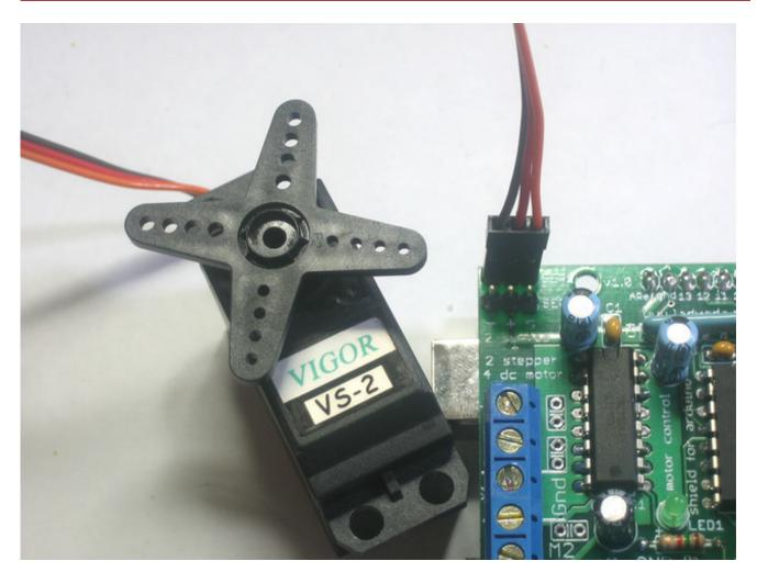
Hobby servos are the easiest way to get going with motor control. They have a 3-pin 0.1" female header connection with +5V, ground and signal inputs. The motor shield simply brings out the 16bit PWM output lines to two 3-pin headers so that its easy to plug in and go. They can take a lot of power so a 9V battery wont last more than a few minutes!
