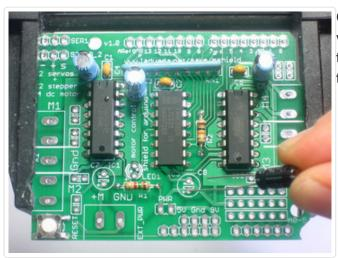
Capacitors are not color-coded. The body color can vary from blue to violet to green to black sobe sure to read the value on the side, don't depend on the color!
