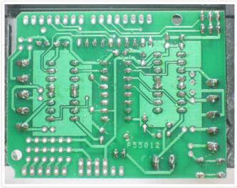
Next, place the 8-pin and 6-pin headers into the Arduino board. This will make sure that the headers are perfectly lined up. Make sure the Arduino is not plugged in or powered!
