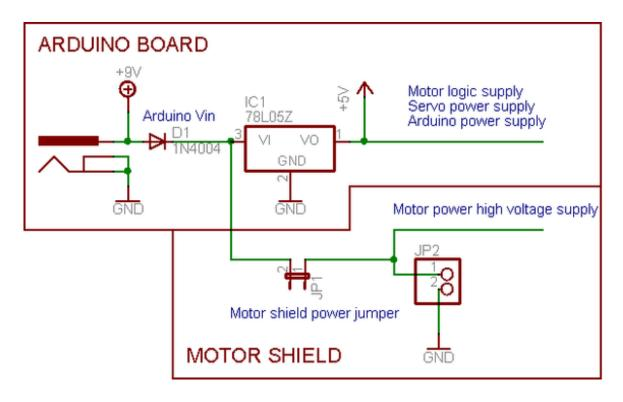
If you would like to have a **single DC power supply for the Arduino and motors**, simply plug it into the DC jack on the Arduino or the 2-pin PWR\_EXT block on the shield. Place the power jumper on the motor shield.
