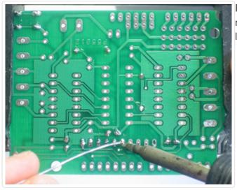
Flip the board over and solder in the resistor network and switch. You won't need to clip the leads as they are quite short aleady.
