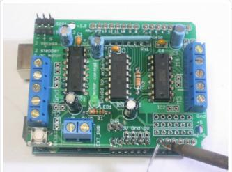
Solder in each pin of the header.
