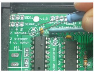
capacitors **C1**, **C3**and **C5**. Electrolytic capacitors are polarized and must be placed in the correct orientation or they could pop! The long leg of the capacitor is the positive (+) leg and goes into the hole marked with a +. The close-up images shown here indicate with hole is the + one.
