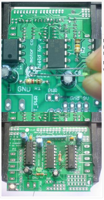
Next is the 3mm LED used to indicate motor power. LEDs are polarized, just like capacitors, and the long lead is the positive (+) lead.
