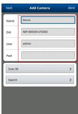
**Three**: Input the UID on the "Device ID" of the Android APP. The default username is: admin.No password.Note:the "Device ID" is on the bottom of the ip cameras.
