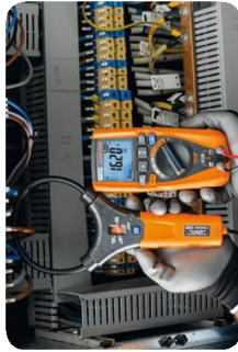
AC current measurement with flexible transducer F3000L.
