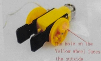
3 Use the "E" screw to install the Yellow wheel on the motor
