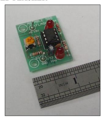
Finally, connect a battery or power supply between 5V and 15V DC to the pins. The LEDs should start to flash off and on.
