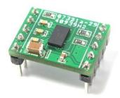
This is a breakout board for Freescale's MMA7361L three-axis analog accelerometer. The sensor requires a very low amount of power and has a g-select input which switches the accelerometer between  $\pm 1.5$ g and  $\pm 6$ g measurement ranges. Other features include a sleep mode, signal conditioning, a 1-pole low pass filter, temperature compensation, self test, and 0g-detect which detects linear freefall. Zero-g offset and sensitivity are factory set and require no external devices.
