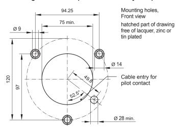
Reduced scale diagrams / dimensions in mm
