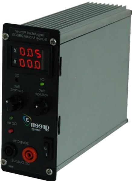
This Module is a variable output Power Supply Module. Takes up 1 slot in a Casing.
