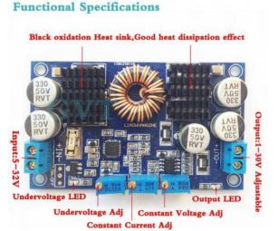
This product is an adjustable power with under-voltage detection threshold. It is designed to withstand maximum output current of 10 A, and can continuously dissipate 80 W up to 130 W, when the heat dissipation is improved. ADDITIONAL HEAT SINK TO BE ADDED IF USED ON MAXIMUM POWER
