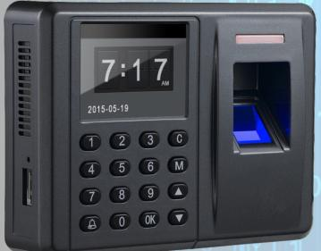
The SPARROW reader has fingerprint, RFID card and pin password functionality. Ideal for SME's with a user capacity of 1000. It can do a basic one door access control application or if configured with the Amatec WOLF controller it will have a fully functional access control system.
