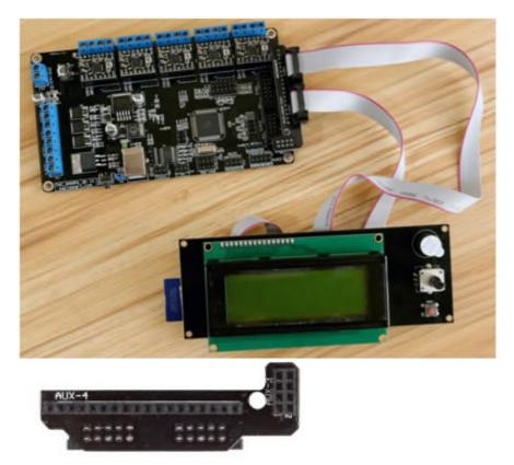
If you want to install an all in one LCD/SD module use the supplied adapter to ensure that the SD card reader works. If you only use the ribbon cabled plugged directly into the board it will not include the SD card pins (see point 12).
