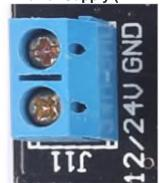
For 12v supply ensure you use more than 10A otherwise the board may not function correctly. 16A-18A (500w-600w) is recommended.
