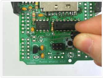
Next are the three electrolytic capacitors **C1 C4** and **C9**.
