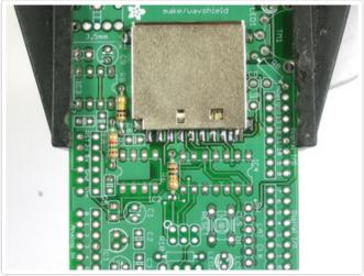
Finish up the resistors by placing **R8** (100Kohm), and **R7** (1.5K)
