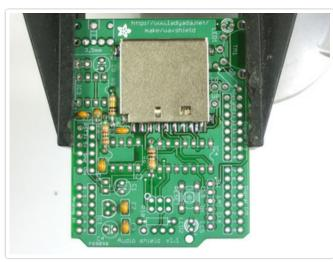
Once you're sure you have **C8** correct, you can place the remaining 0.1uF ceramic capacitors **C2, C3, C5, C6** and **C7**.
