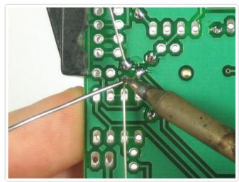
Solder and clip the small capacitor leads.
