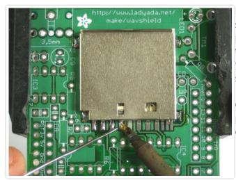
Now go thru and solder the 8 leftmost pins that stick out from the holder. The three rightmost pins are thinner and closer together so they are tougher to solder. Luckily they are not used and you simply skip them (although the photo shows them done).
