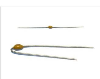
Next is the 0.01uF ceramic capacitor **C8**. The tricky part here is that in older kits there are many 0.1uF ceramic capacitors in the kit that look identical to the 0.01uF!
