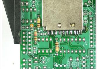
Ceramic capacitors are non-polarized and can go in 'either way.'
