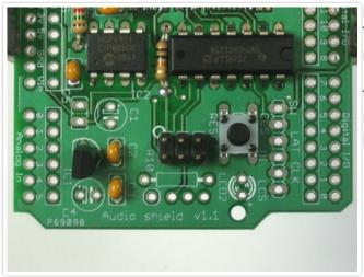
Next is the reset button and the ICSP header. These let you reset the Arduino manually, and reprogram it directly with a AVR programmer.
