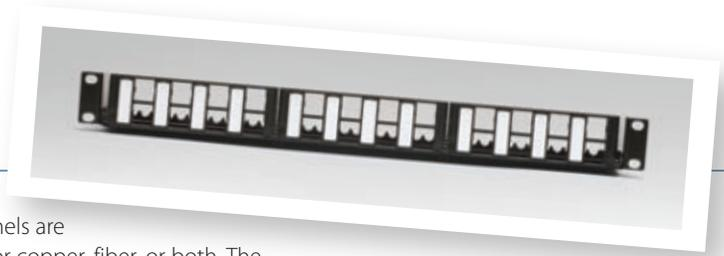
The SYSTIMAX GigaSPEED X10D M3000 Modular Patch Panels are patch panels for M-series outlets that can be configured for copper, fiber, or both. The M3000 is a 24-port panel and can mount in a 19-inch (483 mm) rack with universal hole spacing.
