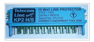
A high speed plug-in card to interface with standard Krone LSA plus disconnect blocks. Offering minimal insertion loss and near end crosstalk, these cards are ideal for large structured wiring installations up to 10Mbits/sec. Each card protects five 4 wire circuits. A new earthing system ensures a high degree of protection.
